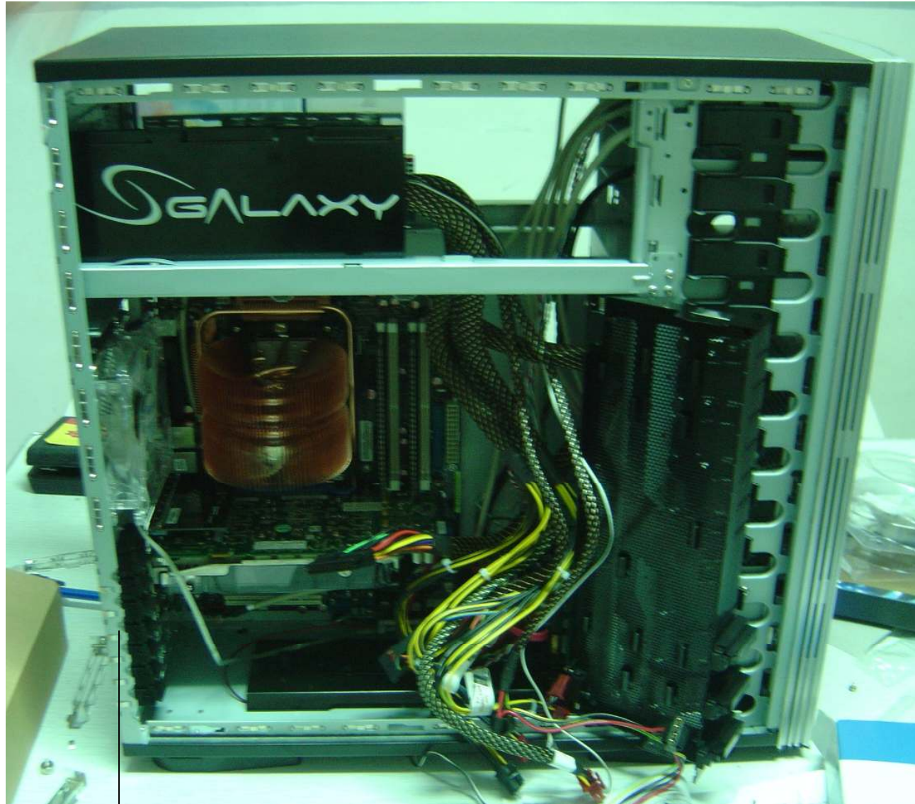
Side view of Pc after all the components had been installed and wired together
